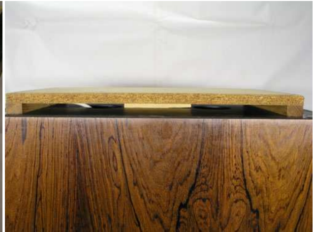
Base plate covering two bottom holes of 54 mm diameter. Apparently no feet was ever attached to these speakers. Some small rubber or felt pads would do well in stabilising the speaker on the floor. A DIN socket is seen at the end of the base plate for connecting to the amplifier. I removed this and added a pair of heavy screw connectors.
