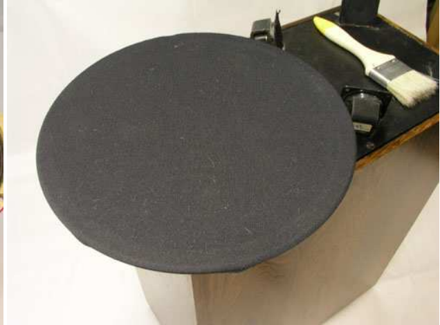
Left: Two renovated 9710 drivers, i.e. cone suspension added a thin layer of flexible coating. Right: I rarely have to sew making loudspeakers, but this calls for a stocking of front grille cloth as the drivers pointing upwards are true dust collectors.
