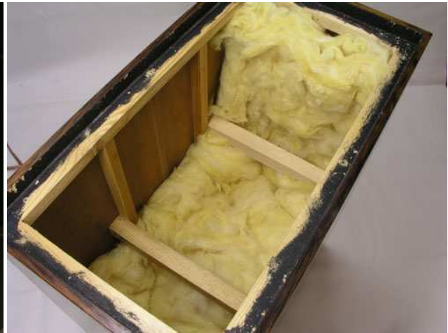
Right: Damping material dividing cabinet into two sections.
