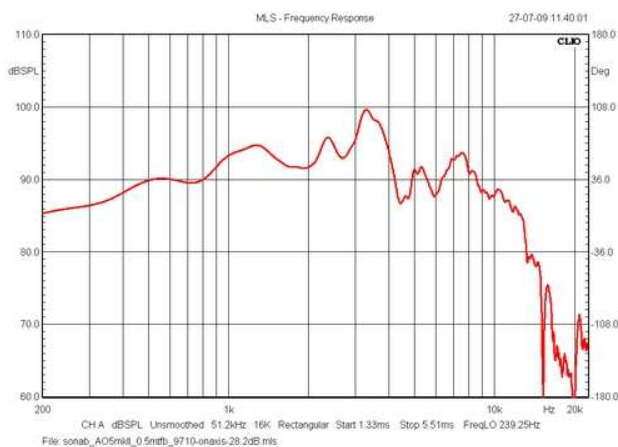
Here a measurement on-axis, 0.5 meter distance normalised for 2.8V/1 meter. System sensitivity is around 90 dB/2.8V/1m valued from the response @ 500 Hz.
