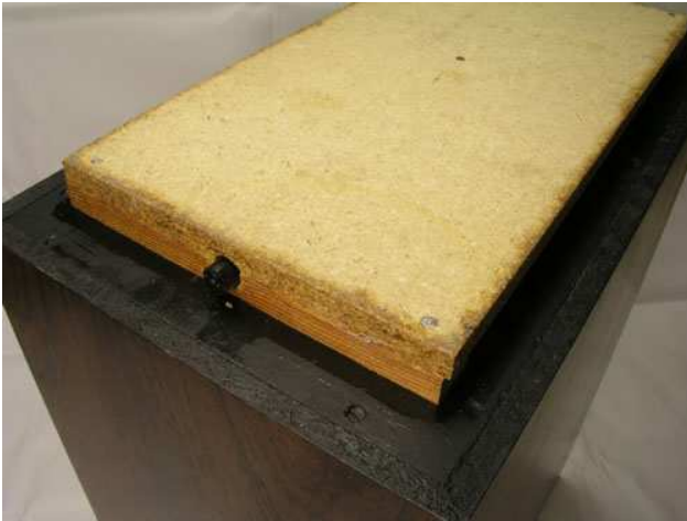
Base plate covering two bottom holes of 54 mm diameter. Apparently no feet was ever attached to these speakers. Some small rubber or felt pads would do well in stabilising the speaker on the floor. A DIN socket is seen at the end of the base plate for connecting to the amplifier. I removed this and added a pair of heavy screw connectors.
