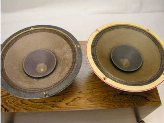
Left: Two renovated 9710 drivers, i.e. cone suspension added a thin layer of flexible coating. Right: I rarely have to sew making loudspeakers, but this calls for a stocking of front grille cloth as the drivers pointing upwards are true dust collectors.
