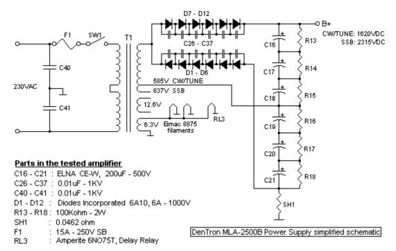
Some of the measurements shown, should be taken with some caution, as this amp has other type of filter capacitors in the high voltage supply than delivered from the factory. The stiffness of the mains used should also be taken into account.
