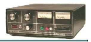
As seen from the measurements previously made, the MLA-2500B has a very high transformer- and filament inrush current which should be reduced. It can be reduced by using a properly designed Step-Start. It's also a good idea to optimize the filament voltage to increase the lifetime expectancy of the tubes.
