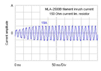
Filament inrush current with 150 Ohm current limiting resistor.
