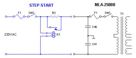
R1 : Current limiting resistor K1 : Time-Delay relay
