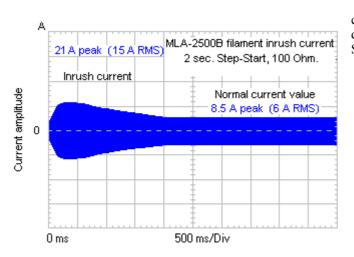
current. As seen, the filament inrush current is decreased from 37A RMS to 15A RMS. The Step-Start used has a 2 seconds duration.
